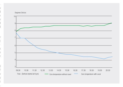
We aimed at keeping the same return-air-temperature in both islands and were successful. The average retur-air-temperature in the open island was  $+3.81^{\circ}$ C and  $+3.91^{\circ}$ C in the island covered with heat reflective glass. The core temperature of the refrigerated food was checked every half hour from 9:30 am until 9:00 pm. Defrosting of the refrigerated island began at 8:00 pm.
